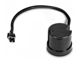
The P2.0 Position Control is a microprocessor position feedback control providing a 0 -10 volt DC output indicating actuator travel. The control uses two inductive pulse count sensors and a counting wheel to accurately determine actuator position. A third sensor at the full retract position provides a zero or home position indication.
