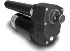
The K2x model provides the highest load rating in its class. This model incorporates all of the base K2 features with a ball nut screw for a 2,200 lb. (998kg) load capability within a compact package size. The K2x includes a bi-directional wrap spring brake for load holding capability. These units are well suited for the most demanding applications where an alternative to hydraulic or air cylinders is needed or where hydraulic power sources are not available.
