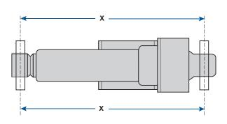
Mounting pins must be parallel to each other as shown above. Pins which are not parallel can cause excess vibration or actuator binding.
