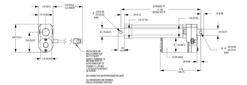
• Stroke and its tolerance are based on a unit with no attached load operating at rated voltage +/-.5VDC, 70°F controlled temperature environment. Note normal wear, temperature changes and load variations all affect the stroke tolerance. If stroke tolerance is critical it is advisable that the selected unit be evaluated for performance in the specific application.
