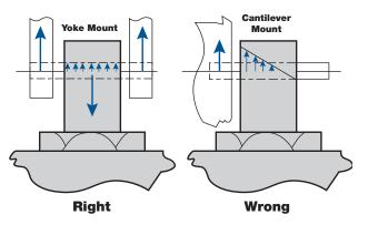
Ensure that mounting pins are supported at both ends. Cantilevered mounting is unacceptable. Failure to provide proper support will shorten unit life.
