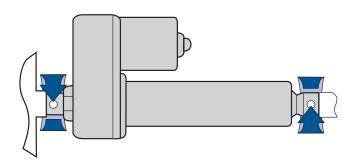
Do not attempt to mount M-Track actuators by the cover tube. The tube is not designed to support the forces required for tube mounting.
