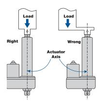
Loads should act along the axis of the actuator. Off-center loads may cause binding and lead to premature unit failure.
